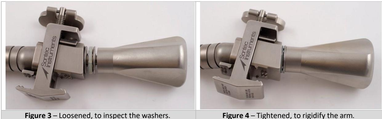
Figure 3 – Loosened, to inspect the washers.
