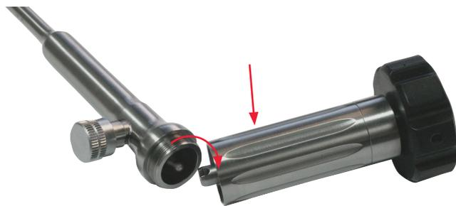
Step 3: Push fan blades down grasp fan below blades and gently twist counter-clockwise to unscrew shaft. Remove shaft from assembly.
